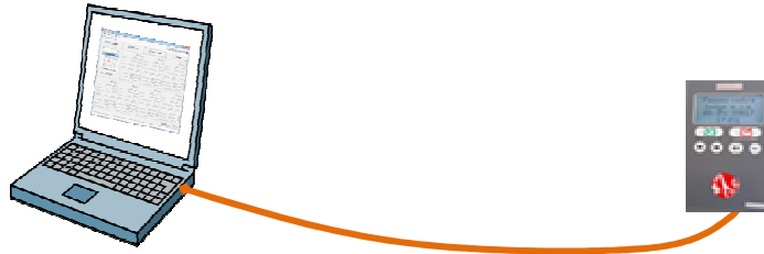
Illustration 10 : Diagram for the connection of a time clock directly to a PC
